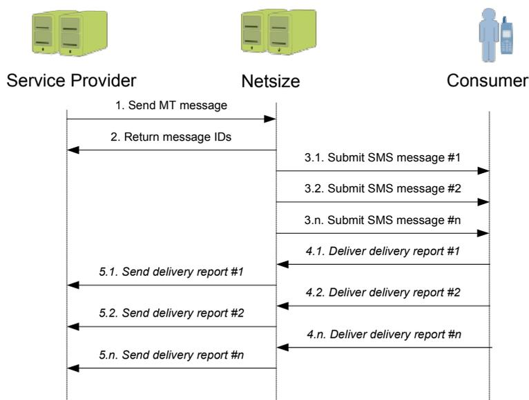
The Netsize system supports the sending of a standard rate SMS message to multiple recipients in a distribution list. The basic flow is described as follows:
